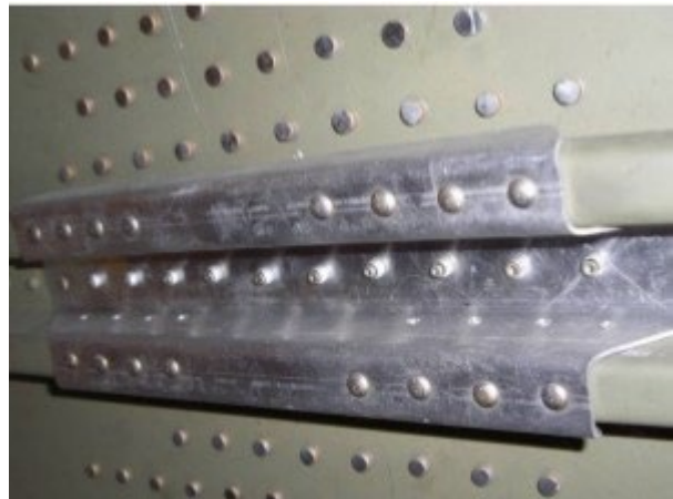
Fig-1: Typical Example of Solid Rivets Installation
