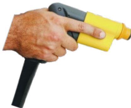
Correct Grip of E-Drill Hand Tool
