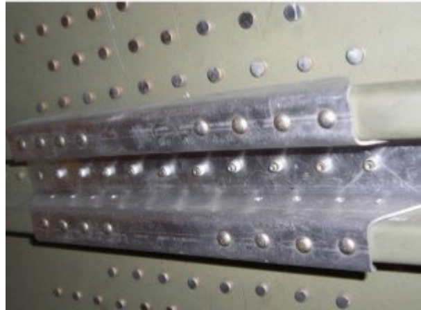
Fig-1: Typical Example of Solid Rivets Installation
