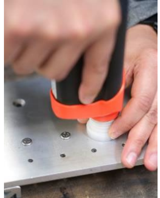
Correct Grip of Button Head Locator
