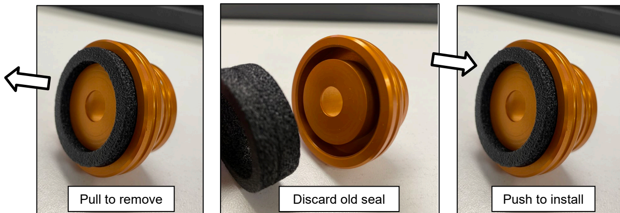
Figure 8. Magnetic Locating Cup Seal Replacement
