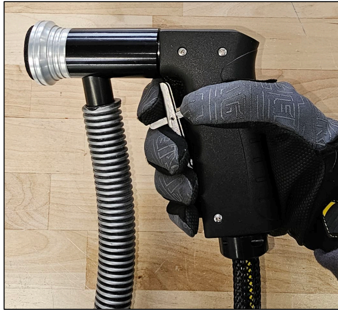
Figure 4. S-Blaster Locked/Vacuum Position
