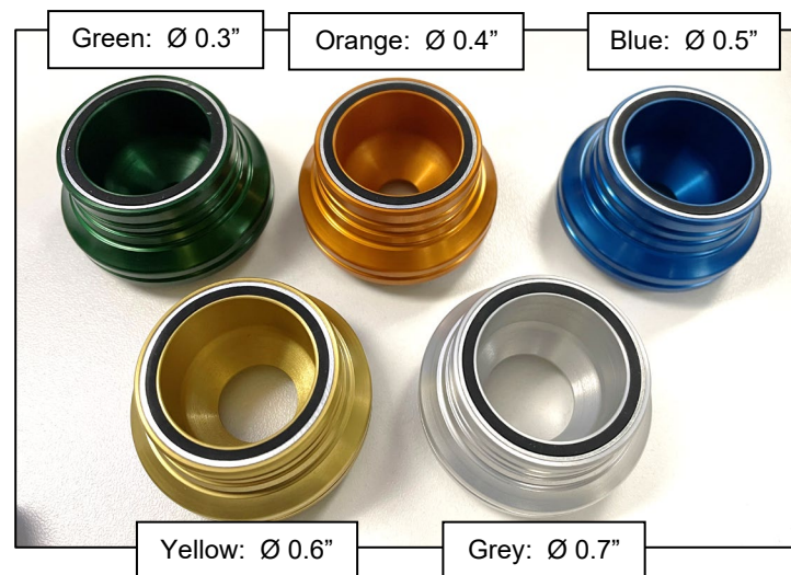
Figure 7. Magnetic Locating/Masking Cups (Hard Mask)
