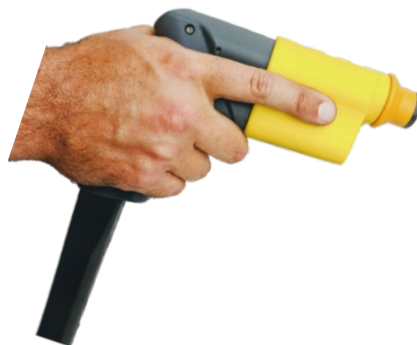
Correct Grip of E-drill Hand Tool
