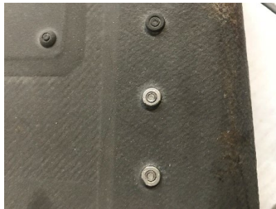
Fig 3- Installed Blind Rivets with Coating Removed
