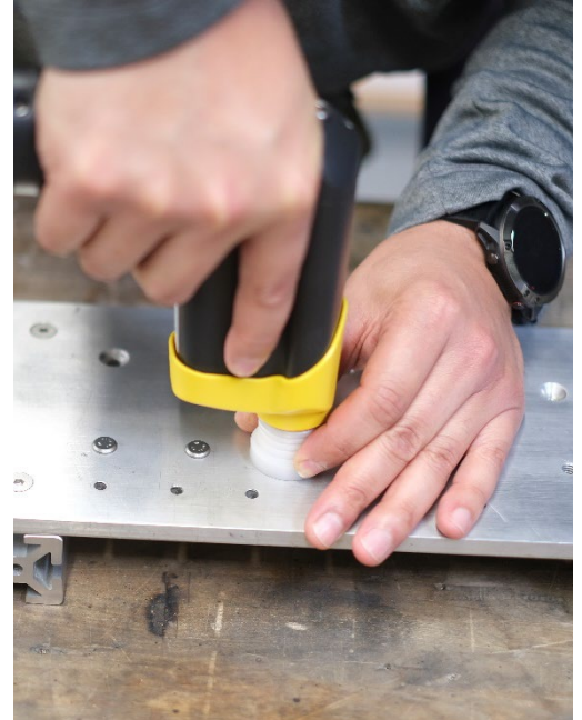
Correct Grip of Button Head Locator
