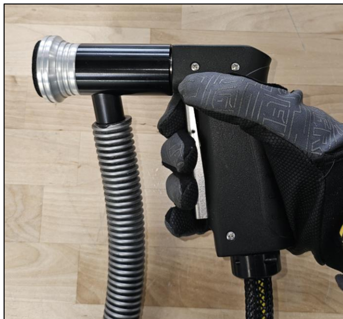
Figure 5. S-Blaster Unlocked/Firing Position
