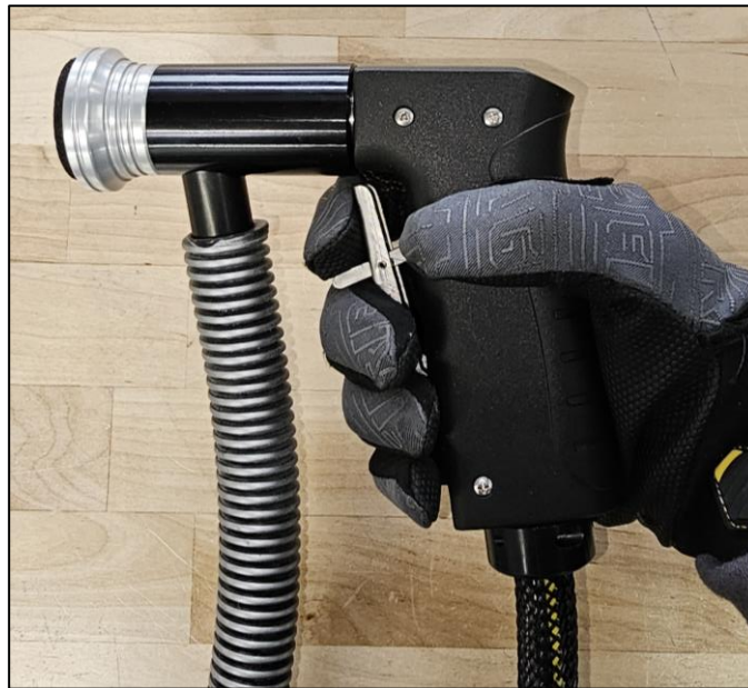
Figure 4. S-Blaster Locked/Vacuum Position
