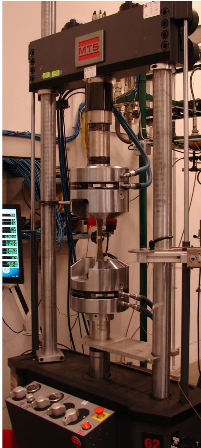
*Figure 1: Fatigue Test Station*
