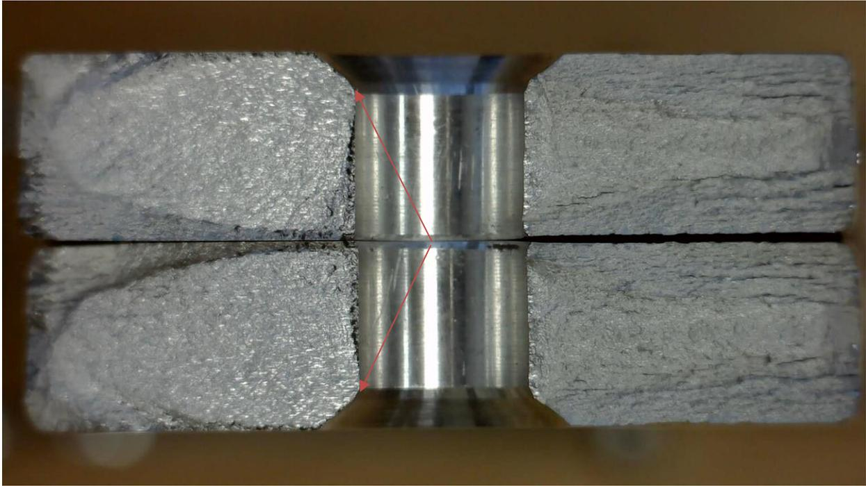
*Figure 13: Specimen BY-13; S, L, CSK failure mode*
