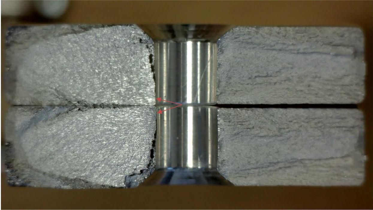
Figure 7: Specimen ECNR-16; S, L, H, P failure mode
