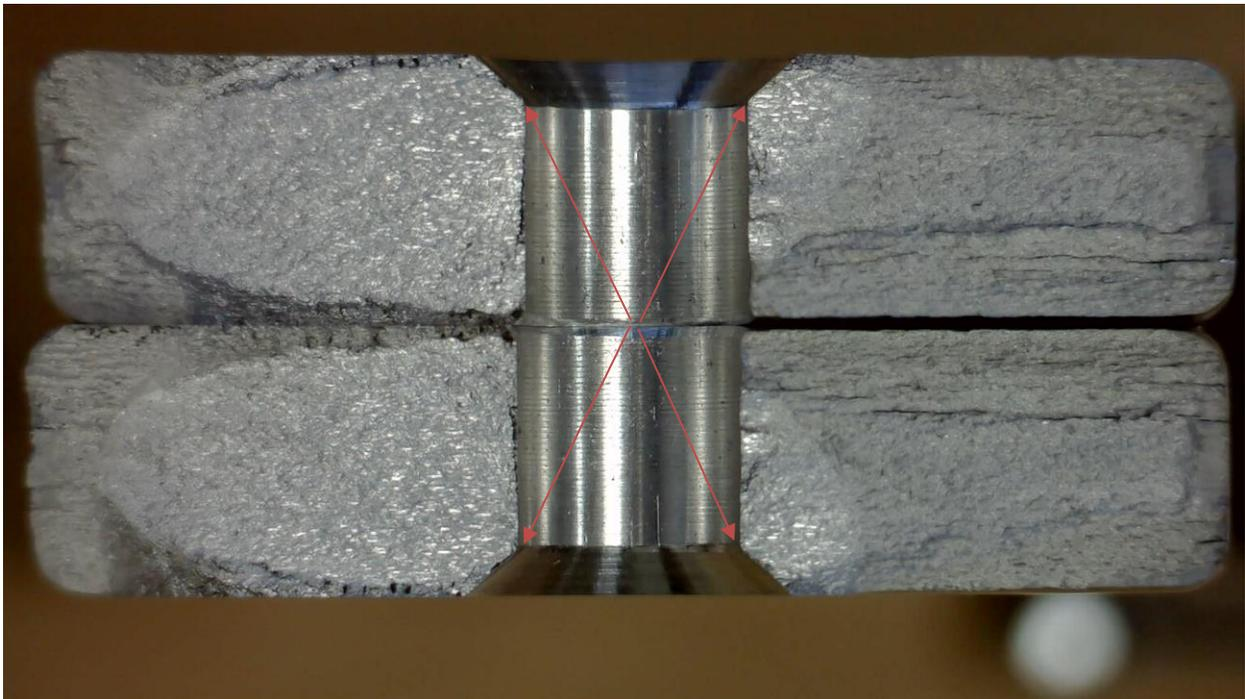
Figure 8: Specimen BX-7; S, B, CSK failure mode
