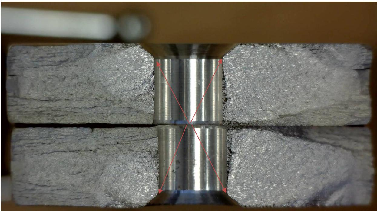
*Figure 12: Specimen XREC-11; S, B, CSK failure mode*
