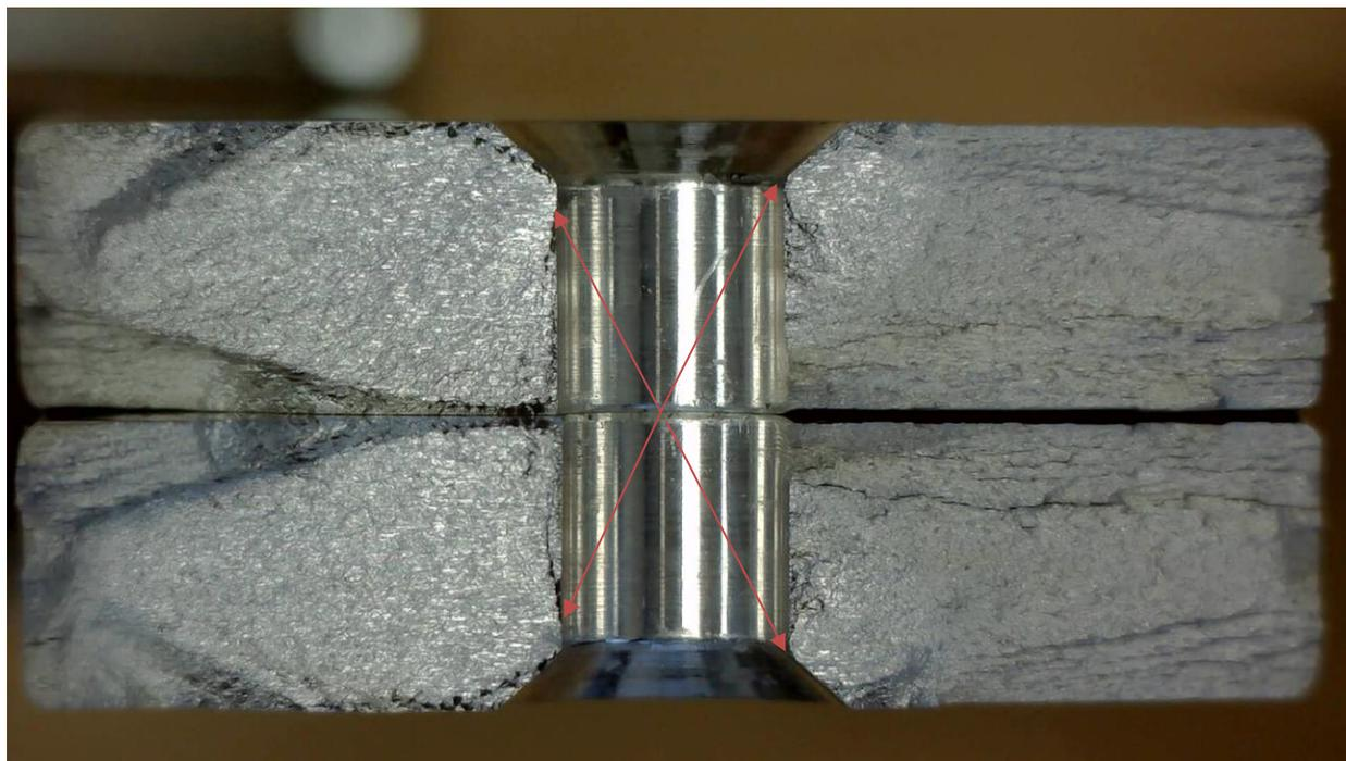
*Figure 6: Specimen ECNR-8; S, L, H / S, R, CSK failure mode*
