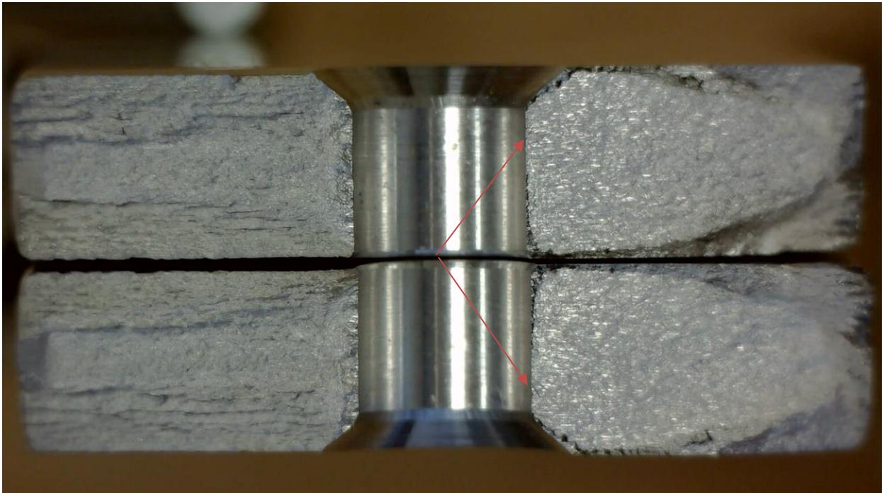
*Figure 14: Specimen BY-14; S, R, H failure mode*
