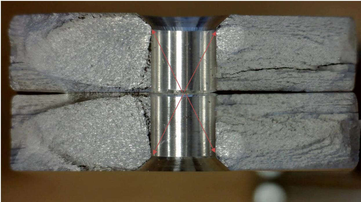
Figure 10: Specimen XREC-7; S, B, CSK, P failure mode
