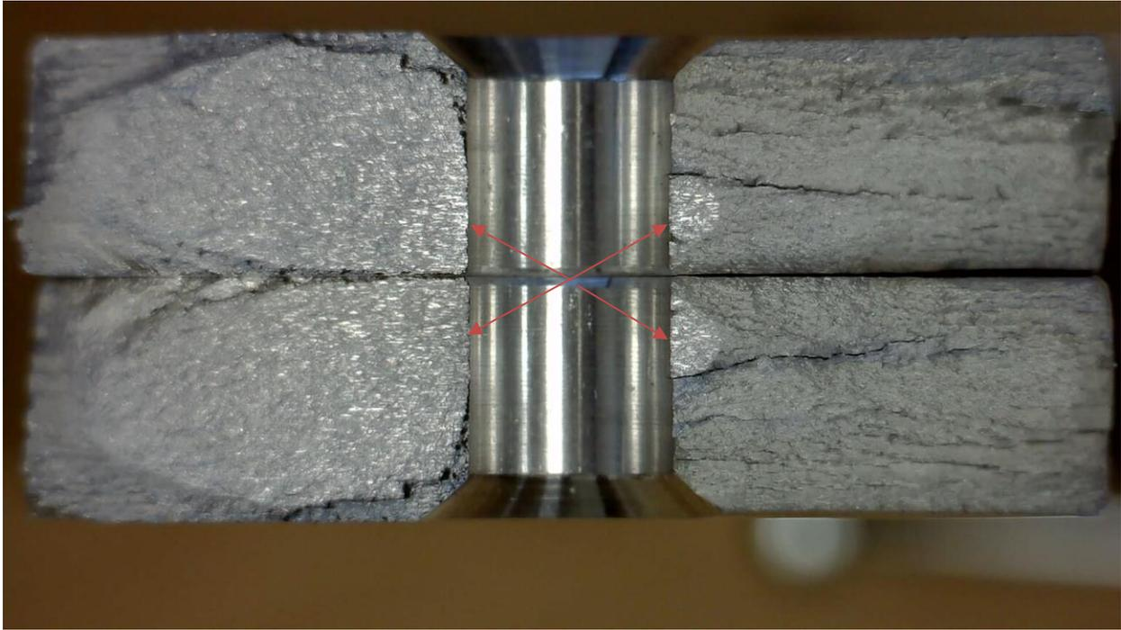
Figure 9: Specimen BX-17; S, B, H failure mode
