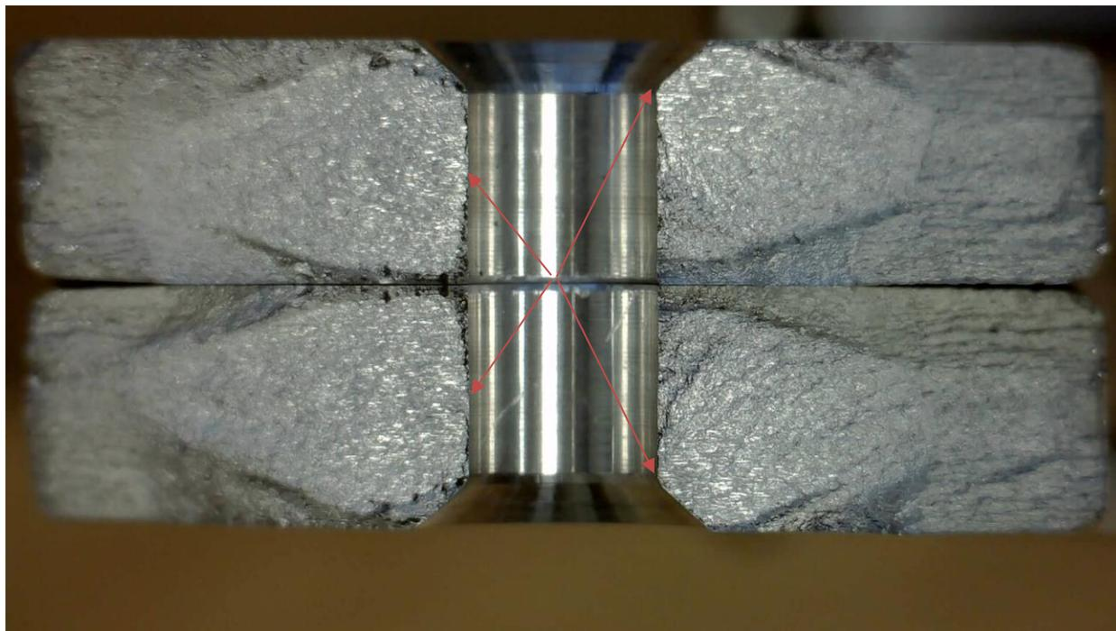
*Figure 5: Specimen NB-9; S, L, H / S, R, CSK failure mode*
