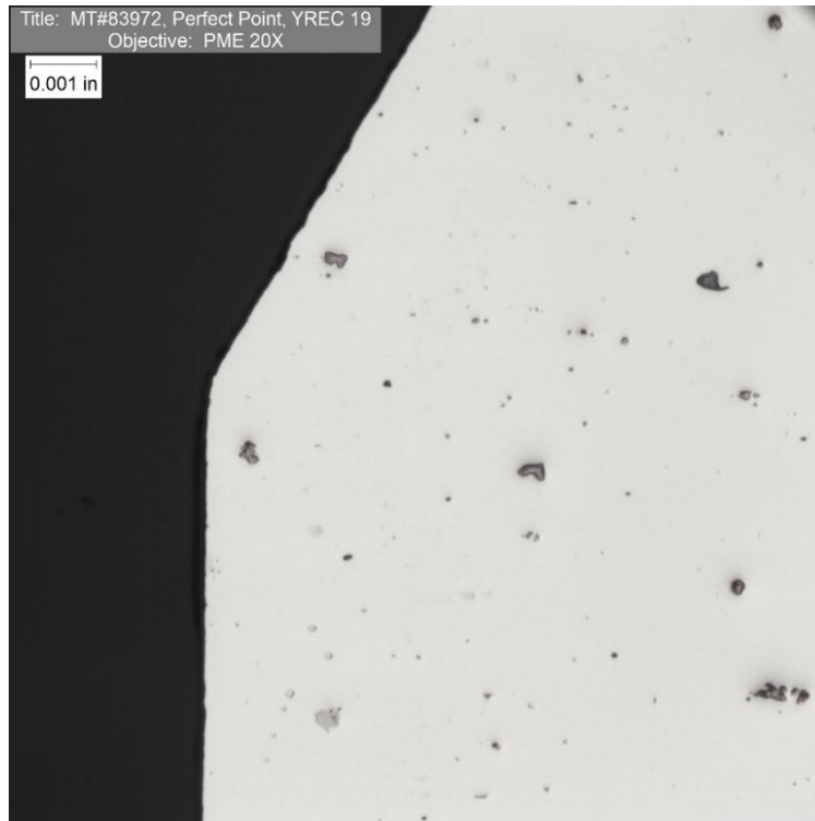
FIGURE 6. MRI Mount No.: 83972. Typical microstructure of the supplied sample YREC 19 is presented in the unetched condition showing the full EDM cut area. No cracking observed. 200X magnification.
