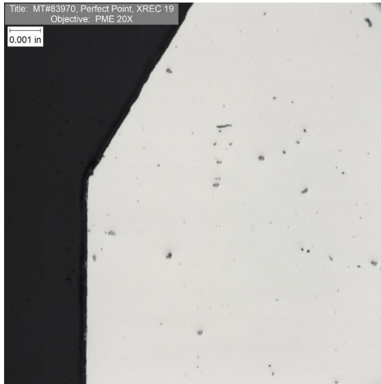
FIGURE 2. MRI Mount No.: 83970. Typical microstructure of the supplied sample XREC 19 is presented in the unetched condition showing the full EDM cut area. No cracking observed. 200X magnification.
