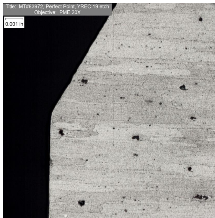
FIGURE 7. MRI Mount No.: 83972. Microstructure of the supplied sample YREC 19 is presented in the etched condition showing EDM cut. No recast layer was observed. 200X magnification, Keller's etch.
