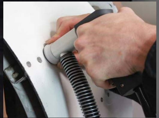
Targeted blast with debris recovery
