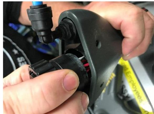
The hand tool case is designed to withstand impacts, but if dropped on its electrode or drive tube mechanism then damage may occur. For this reason, it is always important to keep an electrode and adapter on the hand-tool, even when not in use.
