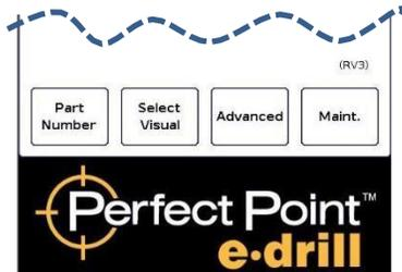
Enter the password provided by Perfect Point, followed by the *enter* button. If the procedure is completed correctly, the Advanced Mode will be enabled. While Advanced Mode is enabled, an **Advanced** tab is visible along the bottom of the screen.
