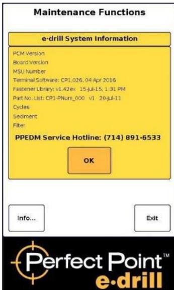
The Informational screen is accessed by touching the “Info” button in the lower left corner of the main maintenance screen. The information screen contains system configuration details and firmware revisions. The screen also contains the **Total Cycles**, **Sediment Tank**, and **Filter** counters.
