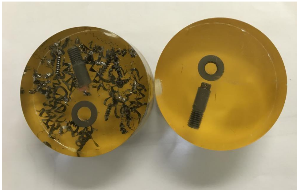
(Fig. 6: Encapsulated FOD Produced by removing One 1/4" Dia. Hi-Lok. Note-E-Drill FST example right-hand side)
