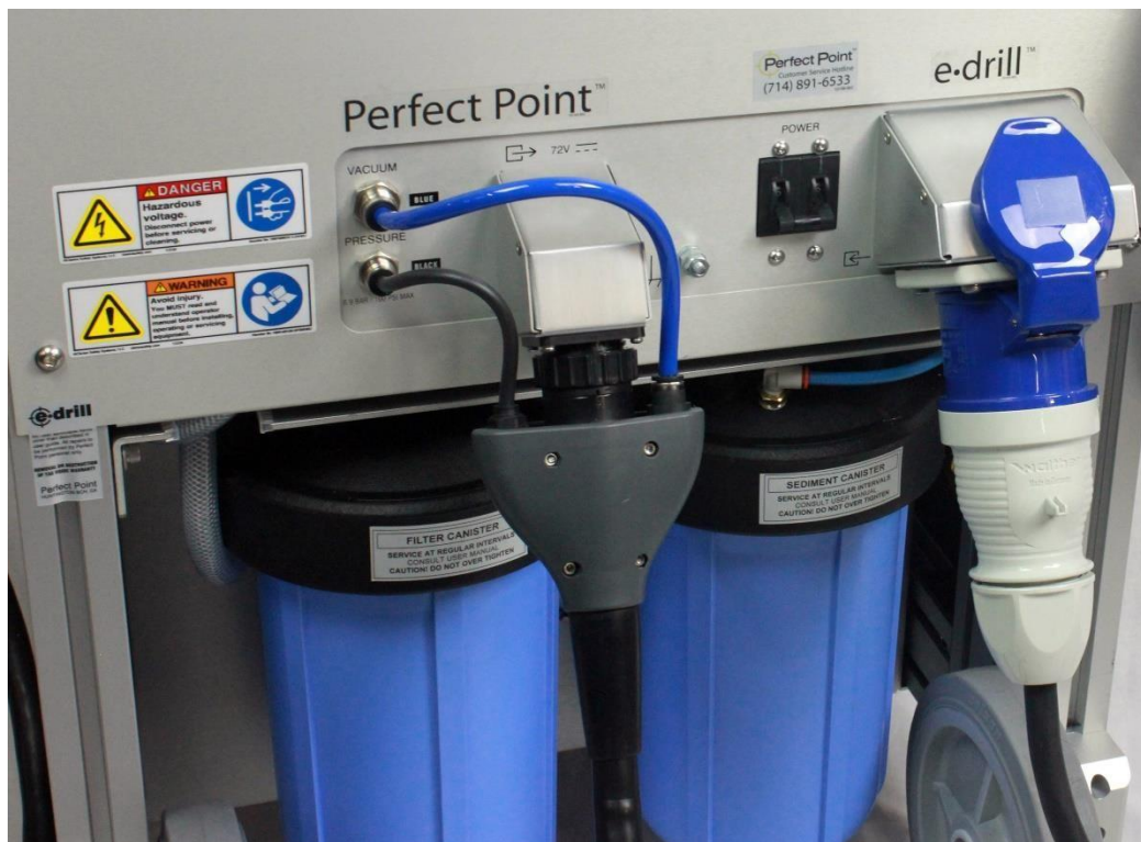
(Fig. 7: Photo of Sediment Collection Tank)
