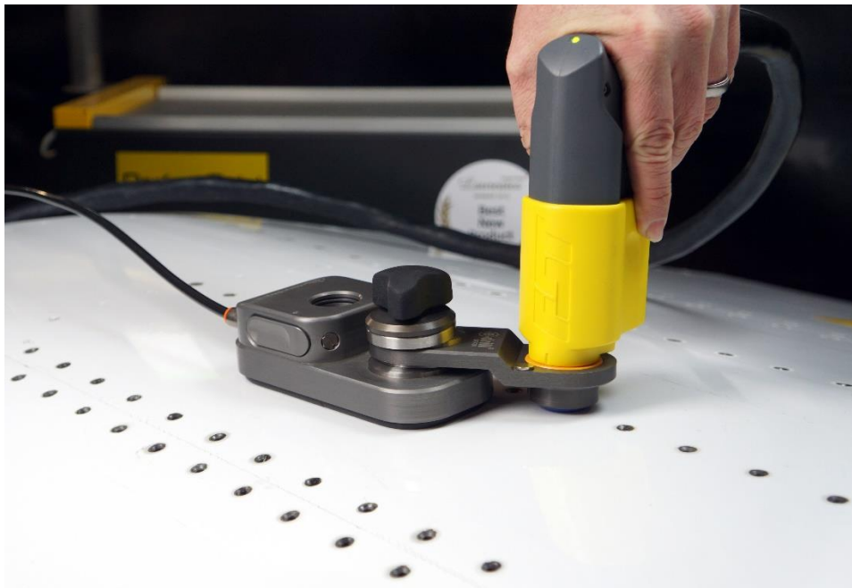
(Fig. 2: E-Drill FST removing Composi-Loks from a wing-skin)
