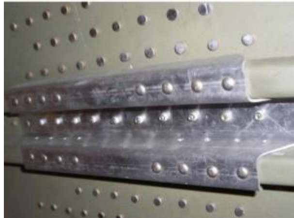
Fig-1: Typical Example of Solid Rivets Installation
