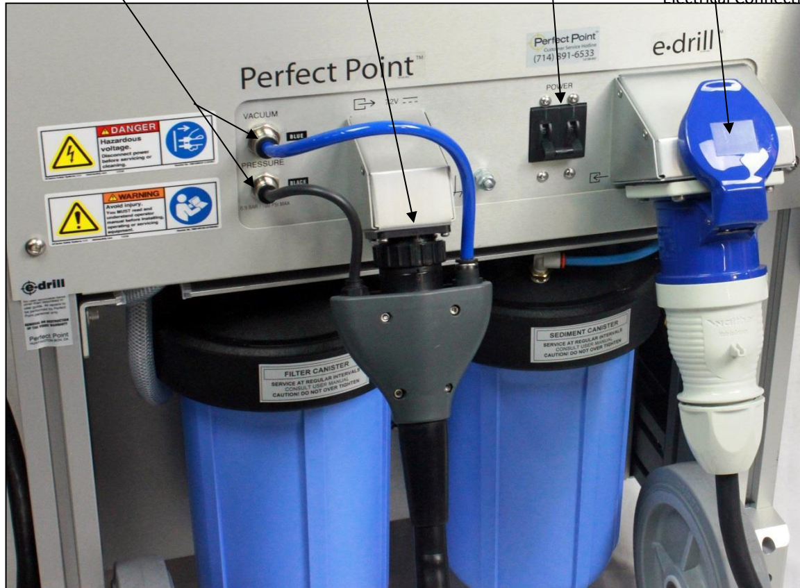
Mobile Service Unit- Rear Connection Panel
