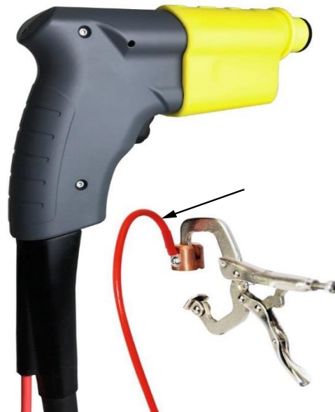
Profile view of EG Hand Tool- note external grounding wire extending from umbilical cable
