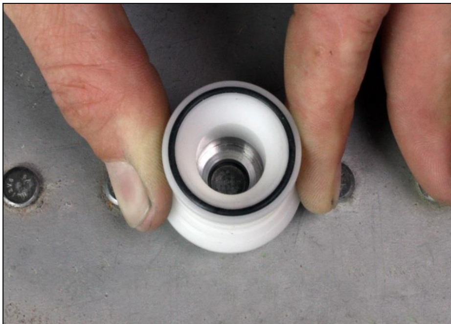
Correct Grip of Button Head Locator
