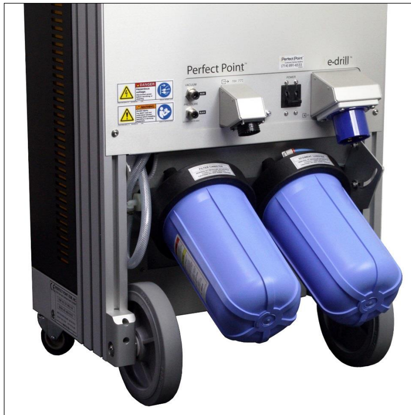
Rear of MSU with Filter Assembly in rotated position
