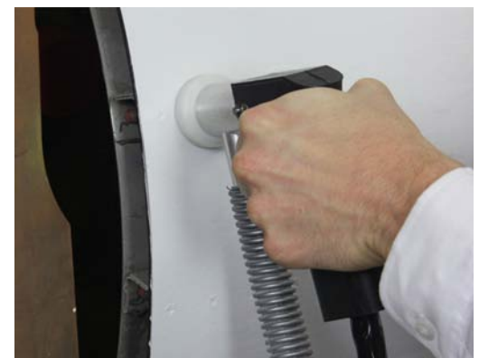
Targeted blast with debris recovery
