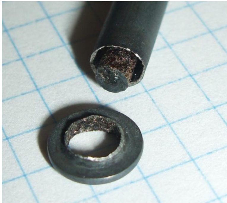
Figure 1. Typical Fastener after removal using the E-Drill process
